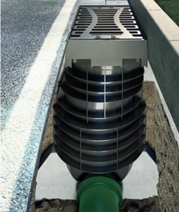
For gutters of parking areas, private car and HGV bypasses, punctual drainage is advantageous. The ACO Combipoint PP road gully, combined together with the Multitop design attachments, provides ideal drainage for parking areas and driving areas. The lightweight gullies are made of plastic and can be rotated, telescoped, shortened and aligned to suit the inclination.
