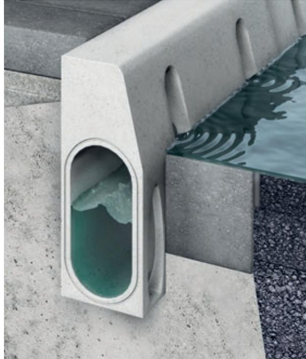
The ACO DRAIN® KerbDrain, a one-piece hollow kerb made of polymer concrete that combines the functions of a kerb and drainage in one component, is suitable for edging areas at car parks. The system impresses with a safe and continuous hydraulic discharge capacity over the entire kerb length.
