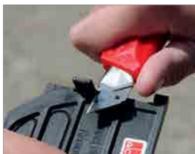
2. Remove Clip A on the left and right with the cutter
