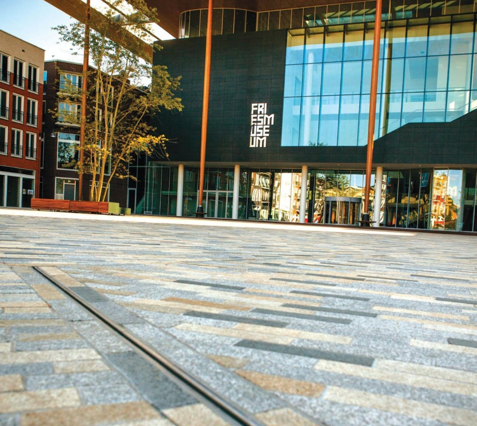
“Hide” or “highlight” are two different approaches when deciding on surface design and drainage. The new SlotTop Strip is the inconspicuous but selfconfident choice. It’s timeless style suits both to historical buildings and modern structures. As an additional feature the width of the outside edge can be customised.
