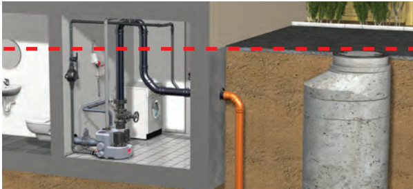
Protection against backflow in gradient to the sewer provided by a wastewater lifting plant in multiple unit dwellings, commercial properties and detached houses with granny flat
