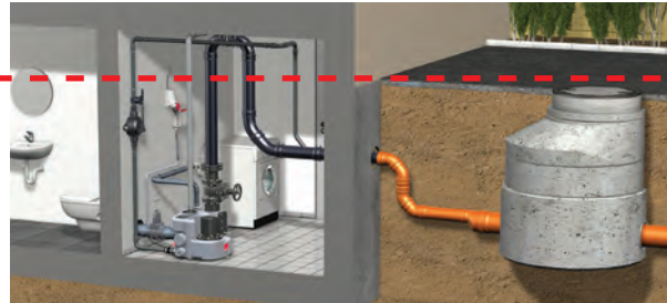
Protection against backflow if the sewer is higher than the sanitary appliances
