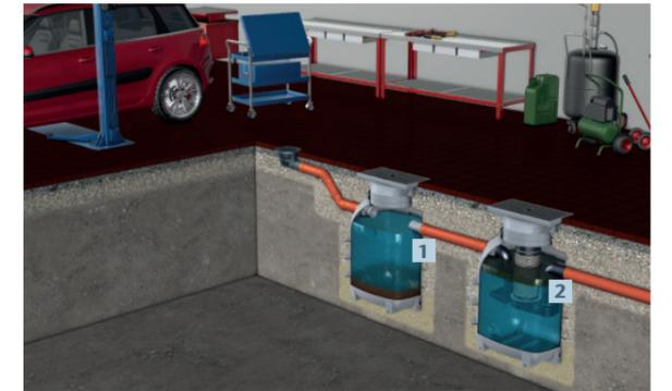
1 Sludge trap 2 Coalisator-P light oil separator
