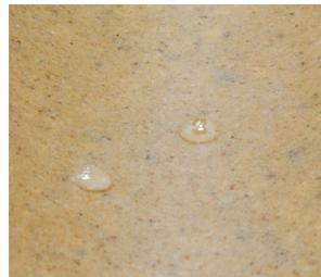
Thanks to **ACO polymer concrete**, a material with a water penetration depth of 0 mm, the entire channel run is watertight.
