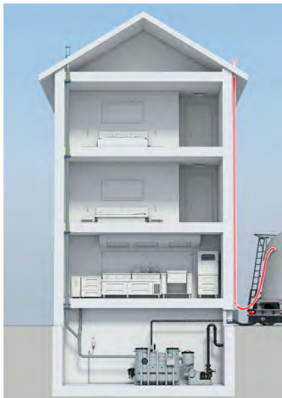
Separate pendulum gas pipe above the roof
