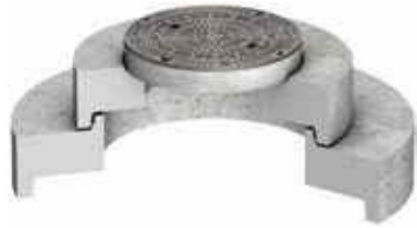
Upper part from reinforced concrete with transition plate and cast iron manhole cover, load class D400 according to EN 124
