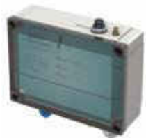
Automatic signaling device with GPS connection and SMS notification
