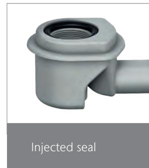
▲ During installation and beyond the period of usage, a permanently tight connection of all components is very important. Therefore, all gully bodies are equipped with a permanently injected seal. This ensures that the seal is not accidentally lost or can slip during installation.
