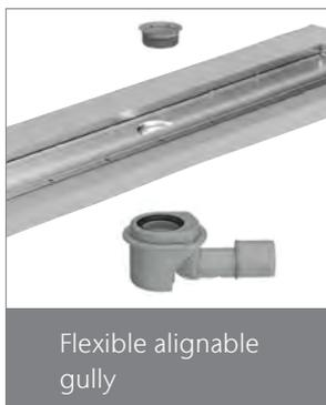
◀ The ACO ShowerDrain M+ can be combined with four different gully bodies to make it suitable for the installation situation. The gully body of the ACO ShowerDrain M+ can be flexibly aligned according to the course of the drainage pipe. Screwed in the middle, the gully body is therefore a secure, force-locked connection that holds the gully securely in position after installation.
