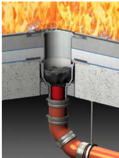
If a fire is present beneath the ceiling, the intumescent mass in the cartridge safely blocks the socket in the drain
